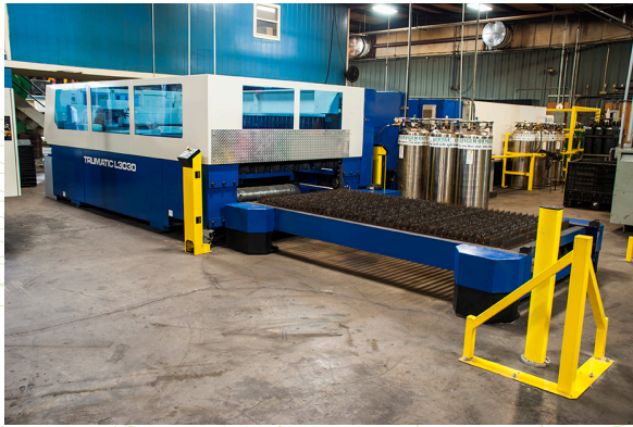
Our laser centers cut up to 1/2" thick steel and 3/16th" thick stainless steel. Shuttle tables accommodate steel sheets up to 60" x 120."
